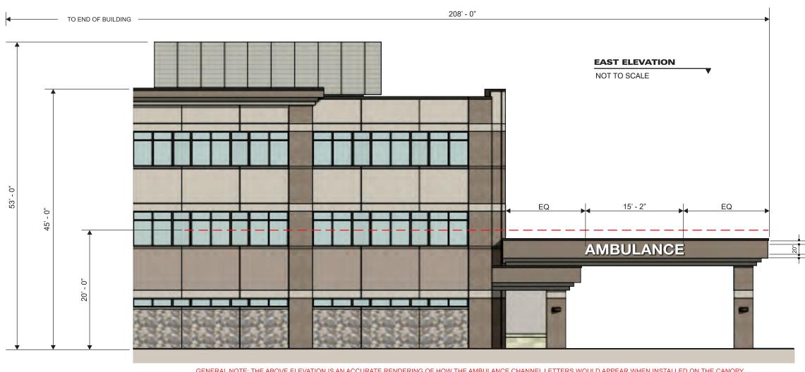
GENERAL NOTE: THE ABOVE ELEVATION IS AN ACCURATE RENDERING OF HOW THE AMBULANCE CHANNEL LETTERS WOULD APPEAR WHEN INSTALLED ON THE CANOPY.
