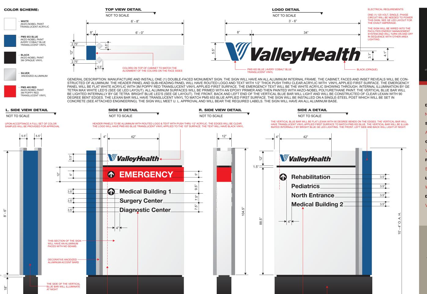
THE SUB-HAEADING PANELS TO BE ALUMINUM WITH ROUTED ARROWS & TEXT WITH PUSH THRU 1/2" ACRYLIC. THE EDGES WILL BE CLEAR. THE TEXT AND ARROW WILL HAVE OPAQUE BLACK VINYL APPLIED 1ST SURFACE.
