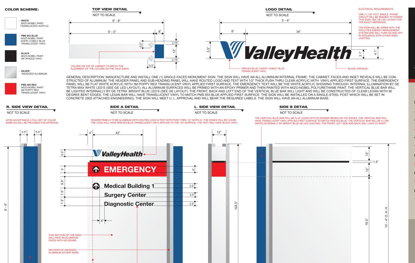
THE SUB-HAEADING PANELS TO BE ALUMINUM WITH ROUTED ARROWS & TEXT WITH PUSH THRU 1/2" ACRYLIC. THE EDGES WILL BE CLEAR. THE TEXT AND ARROW WILL HAVE OPAQUE BLACK VINYL APPLIED 1ST SURFACE.
